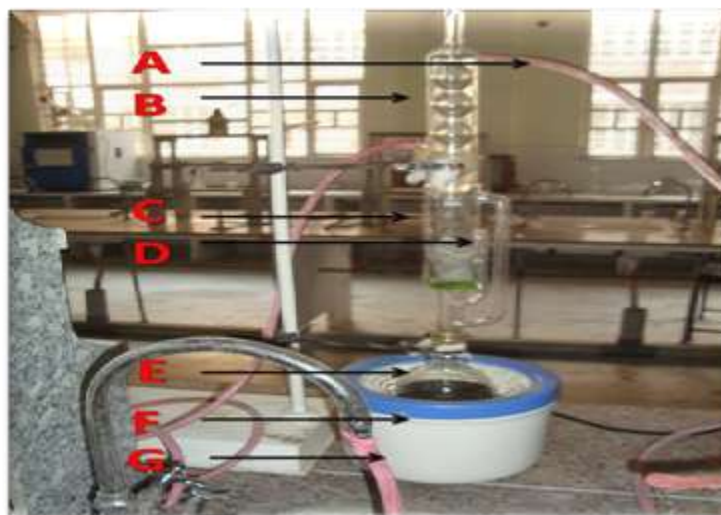
Figure 3: Soxhlet Apparatus ; A- Water outlet, B- Condenser, C-Thimble, D-Siphone tube, E-Round bottom flask, F-Heating mental, G- Water inlet.
