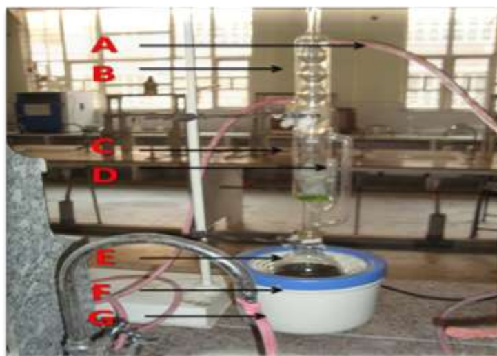
Figure 3: Soxhlet Apparatus ; A- Water outlet, B- Condenser, C-Thimble, D-Siphone tube, E-Round bottom flask, F-Heating mantle, G- Water inlet.
